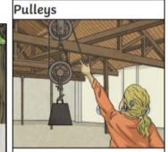
Pulleys can be used to make a small force lift a lighter load. The more wheels in a pulley, the less force is needed to lift a weight.
